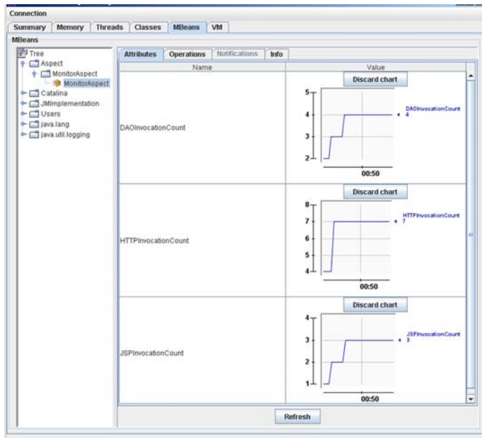
Fig. 7. Data from MonitorAspect is comprehensively visualized as data values change over time, and can be updated in JConsole
